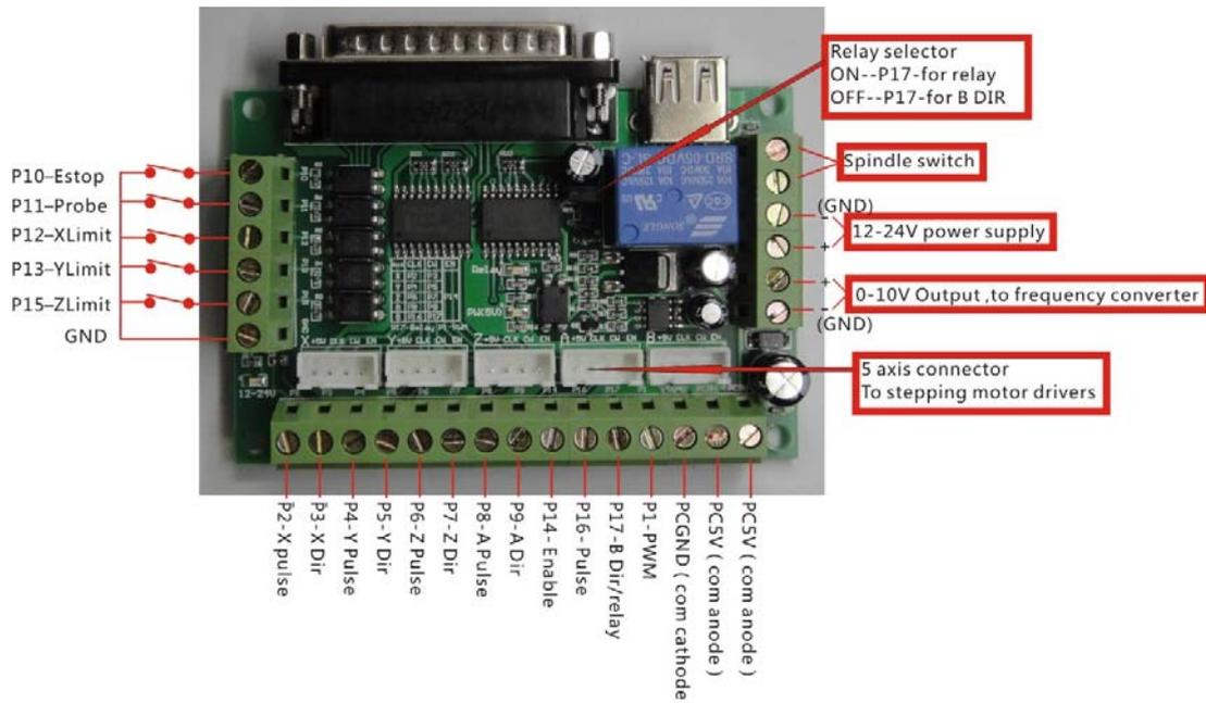
Note: all the settings below is for common anode connection between this interface board and the stepping motor drivers.
