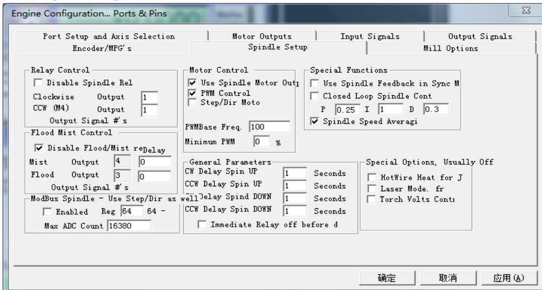
Using PWM to control the spindle speed, also need to set "spindle pulleys" as below:
