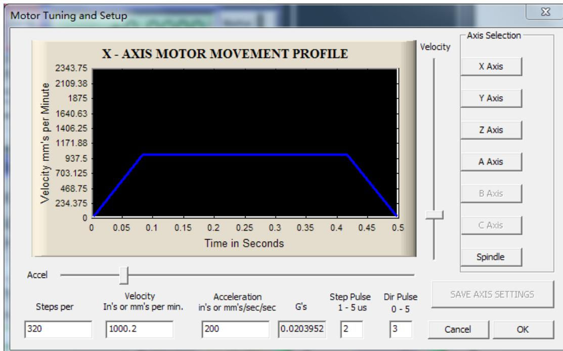
“Steps per” means how many steps it need for moving 1 MM.
