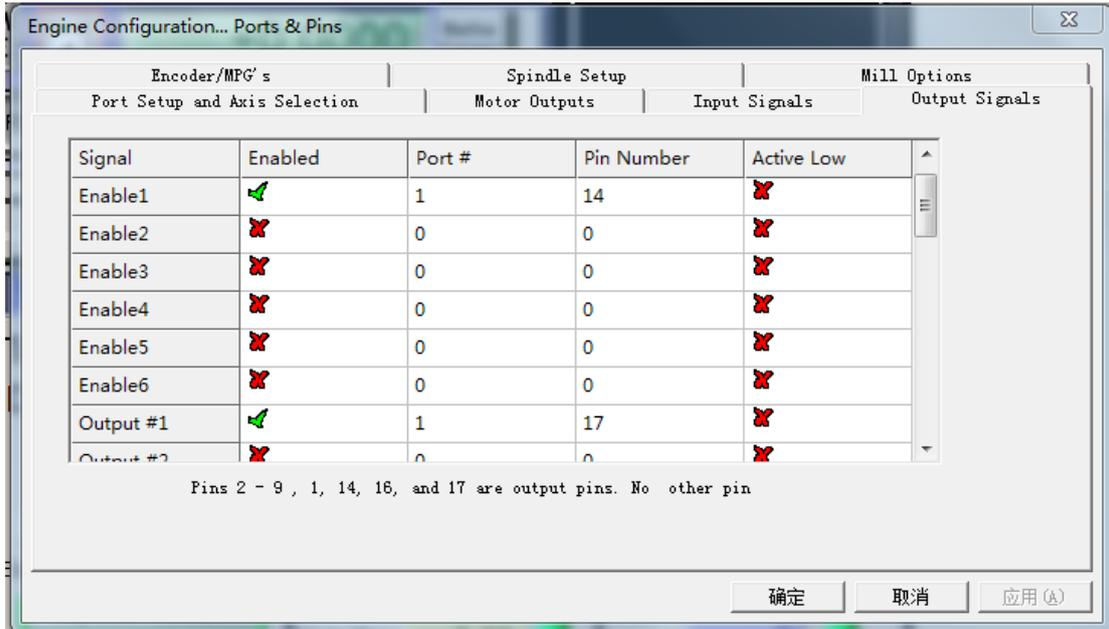
Enable1: setting motor enable setting. --p14
