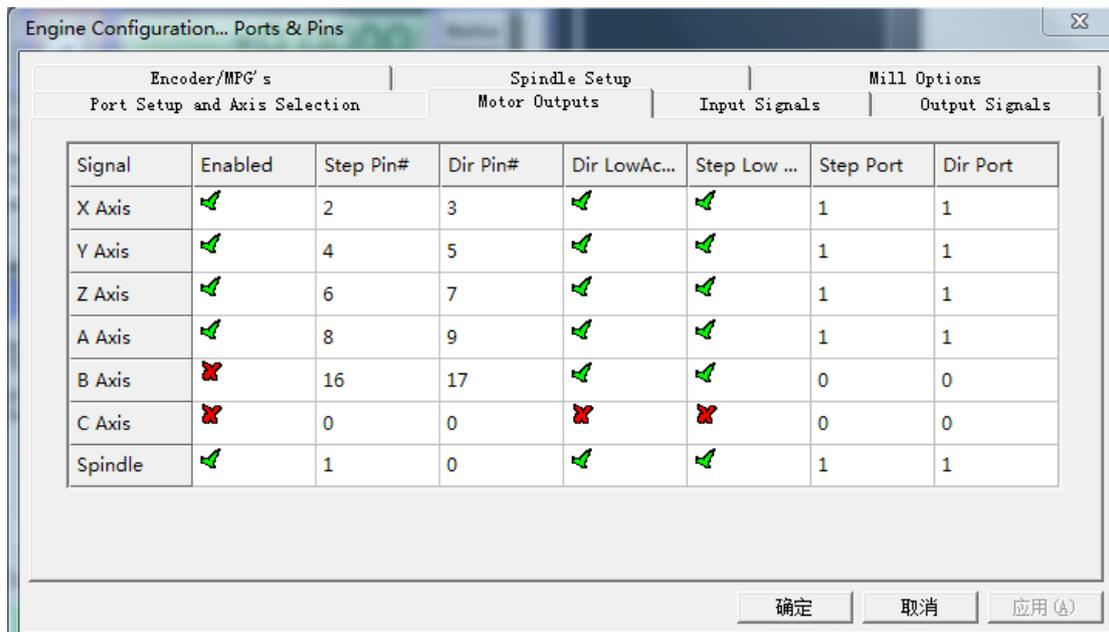
note: the motor turning direction is relevant to its connection , if the direction is not right, you can adjust “Dir LowActive” as on the diagram。
