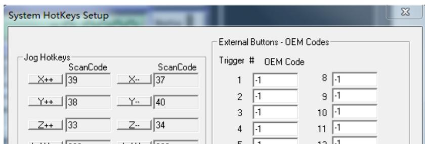
Set the hotkeys of X、Y、Z axis as this diagram, then you can control the motors by this hotkeys on the keyboard.
